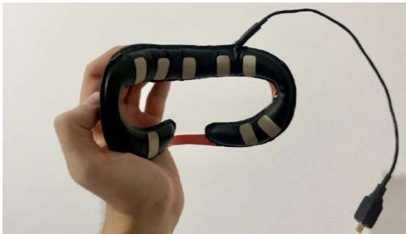
Our device (Standard VR mask with biosensors)
