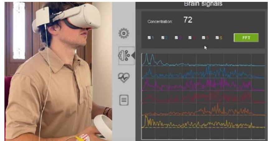
Left side - User wearing the VR mask with biosensors, right side - desktop application for real time monitoring
