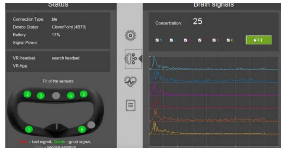
Desktop application for real time monitoring: biosensors connection status, level of concentration, brain signals
